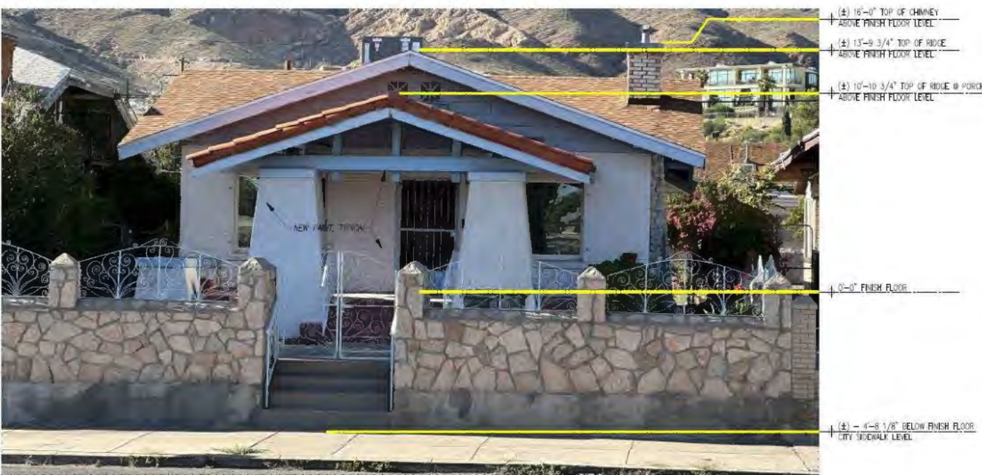
A1 EXISTING FRONT ELEVATION TO REMAIN AS IS N.T.S. EXTERIOR OF EXISTING HOME SHALL BE PATCHED, REPAIR, AND PAINTED AS PER OWNERS SELECTION
