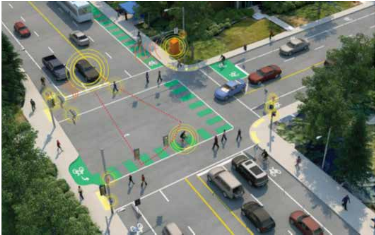
Figure 3.6: Conceptual rendering of a connected intersection where the vehicles, can communicate with the infrastructure as well as with other devices in the area
