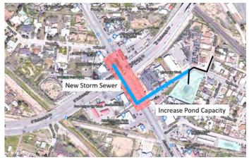
Existing Pond Increase with Storm Sewer Extension Possible Proposed Conditions
