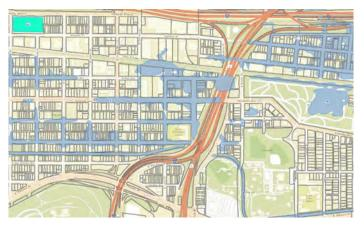
Potential update to the Special Flood Hazard Area along the Alameda Avenue corridor through Chamizal based on the new Preliminary FIRM Maps with an expected effective date in mid 2022.
