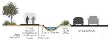
Proposed trail cross-section along canals found in the Paso del Norte Master Plan.
