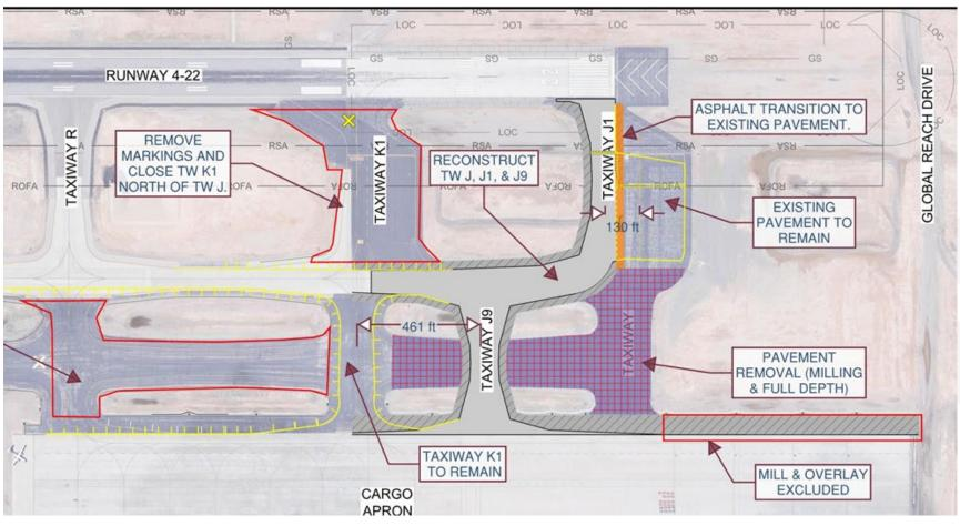
The Airport is installing pavement improvements that will bring the taxiway geometry at the north cargo buildings into compliance with current Federal Aviation Administration (FAA) design standards. Taxiway K2 will be reconstructed and a new Taxiway, J9, will be constructed to replace aging pavement.
