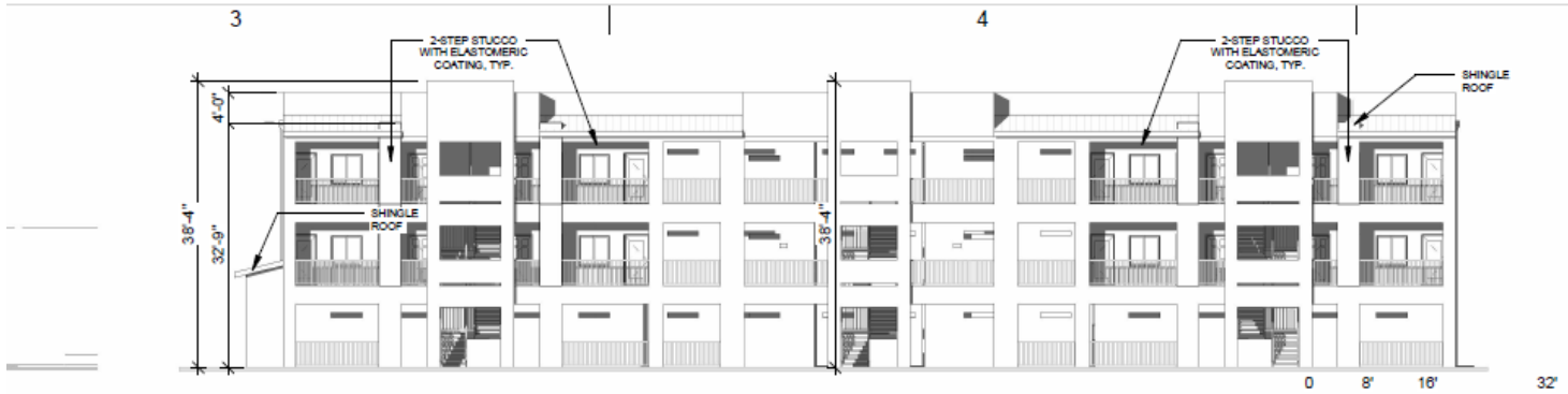
2 BLDG. A - SOUTH ELEVATION 1/16" = 1'-0"
