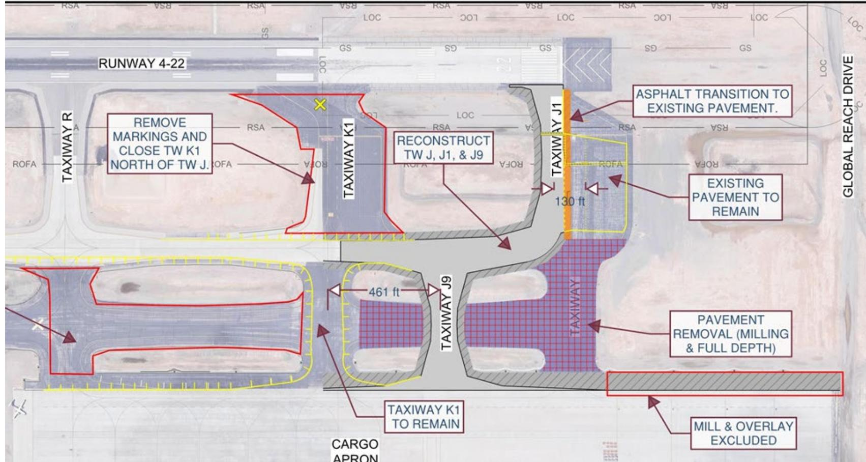
The Airport is installing pavement improvements that will bring the taxiway geometry at the north cargo buildings into compliance with current Federal Aviation Administration (FAA) design standards. Taxiway K2 will be reconstructed and a new Taxiway, J9, will be constructed to replace aging pavement.
