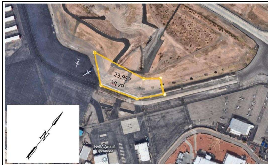
Figure 1 – SIDA Ramp Expansion Approximate Limits
