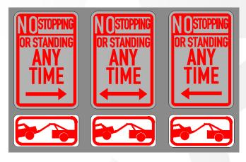
INSTALL "NO STOPPING OR STANDING ANY TIME" R7-4(R); R7-4(LR); AND R7-L) and "TOW-AWAY" R7-201P
