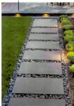
Proposed walkway pavers – 3' x 6' rectangular concrete pavers
