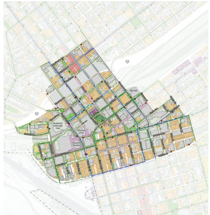
Example of a context and connections map within a ¼ mile from the site's perimeter showing urban design features, transportation infrastructure, and connections. The minimum map scale is 1"=400'.
